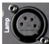
**Lamp** – Plug in a 4-pin gooseneck lamp to illuminate the mixer surface. You can use any industry standard 12V, 5W or lower power lamp. We recommend the Allen & Heath LEDLamp with built-in thumbwheel dimmer.
