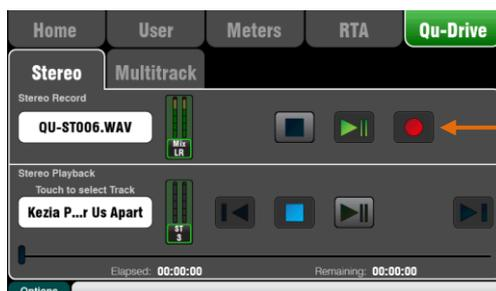
**Stereo Record** – You can record to a USB storage device plugged into Qu-Drive:
