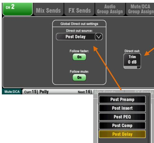
Adjust the channel Direct Output **Trim** from off to +10dB gain. The Direct Outputs can be patched to feed the internal FX devices, for example a delay effect send for a single vocal. They also feed the dSNAKE Monitor outputs (ME Personal Mixing System), and can be set as the CH/ST channel USB source.
