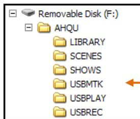
**Copy audio WAV files on to USB** from your computer. Place these in the AHQU / USBPLAY directory. Plug the USB device into Qu-Drive.
