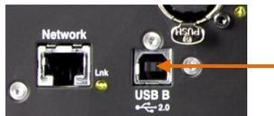
**Connect the Qu mixer to the computer** – Plug a suitable cable into the rear panel USB B port.
