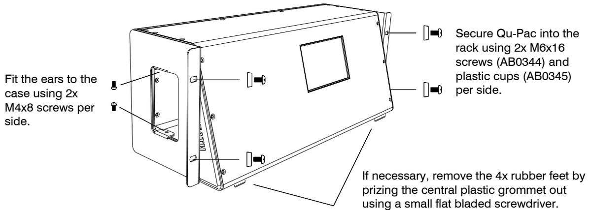
**Note** Allow adequate air flow around the ventilation slots at the rear and through the inside section of the case. Do not block the sides.
