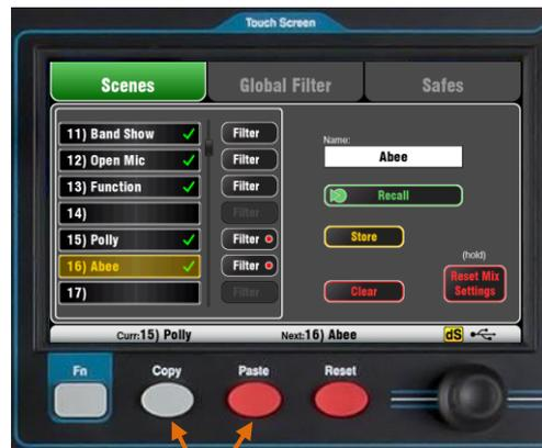
**To Copy a Scene** – Press and hold the Copy key below the screen and then touch the scene to copy. Now press and hold the Paste key and touch the scene in the list to paste to. This copies the scene contents and name.
