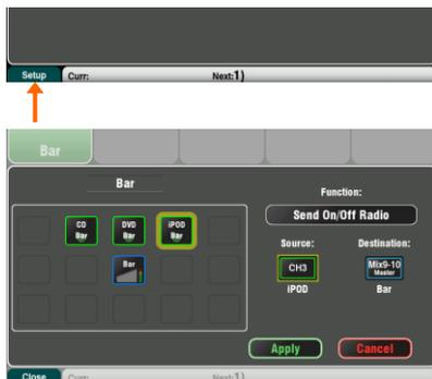
Functions can be assigned to up to 15 positions arranged as a grid of 3 rows with 5 columns. If a position is unassigned then it will appear blank in the user screen.
