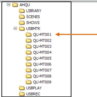
**Note** – We recommend you transfer previous recordings to your computer and then reformat the USB device on the Qu mixer before using it for each show. This will avoid potential audio skipping that may occur with some USB devices containing long recordings.
