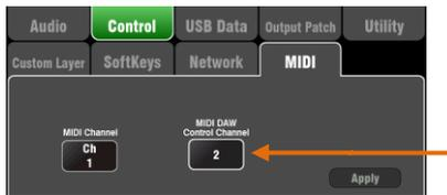
**Set the Qu mixer MIDI channel number** – Use the **Setup / Control / MIDI** screen to set the Qu MIDI channels. Qu DAW control uses its own MIDI channel. This is the next number up from that set for the other Qu MIDI messages. Qu defaults to Channel 1 for standard messages and Channel 2 for DAW control.
