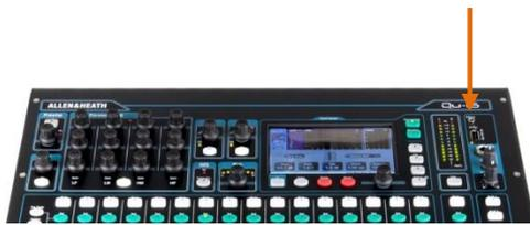
**Note** – Qu-Drive audio recording and multitrack playback require the USB storage device to support high sustained transfer rates. Not all USB devices will guarantee flawless performance.
