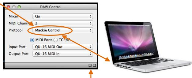
Two squares in the status bar flash to display MIDI I/O activity. To check you are connected to the mixer, the left square should flash when you move any Qu fader.
