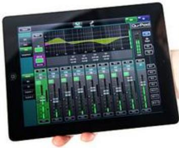
**Qu-Pad** is an engineer's mixing tool giving you the freedom to walk the room or stage and control the sound right where it is needed. Qu-Pad gives you control of the live mix. It is not for system setup or memory management which can be accessed at the mixer. Qu-Pad and the Qu console can work together to provide simultaneous control of independent functions, for example one engineer using the console to mix front-of-house sound, and another using the iPad to mix monitors on stage.
