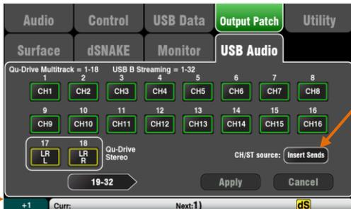
Touch a track box and turn the rotary to select the source. Press the '+1' **Fn** key to increment the assignments. Choose the global source for CH and ST channels and the Audio Groups.
