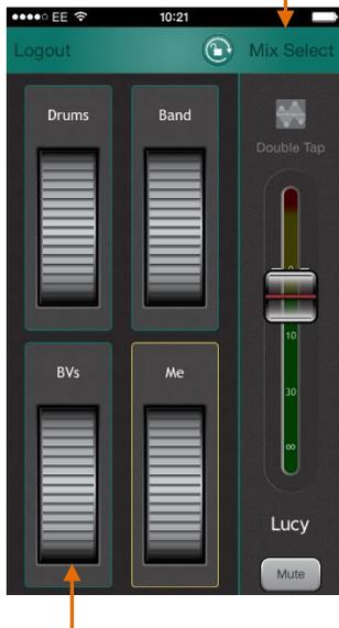
Channels can be assigned to up to 4 local groups, each with its own thumbwheel level control.
