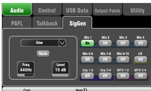
Set up and assign the Signal Generator to test loudspeakers and align levels between equipment.
